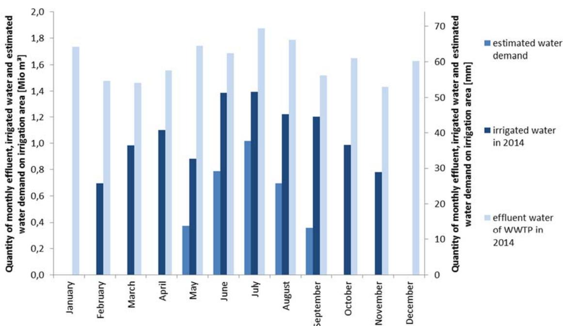
**Figure 17** monthly distribution of effluent water from WWTP, water supply to agriculture and projected water demand in the irrigation area of Braunschweig
