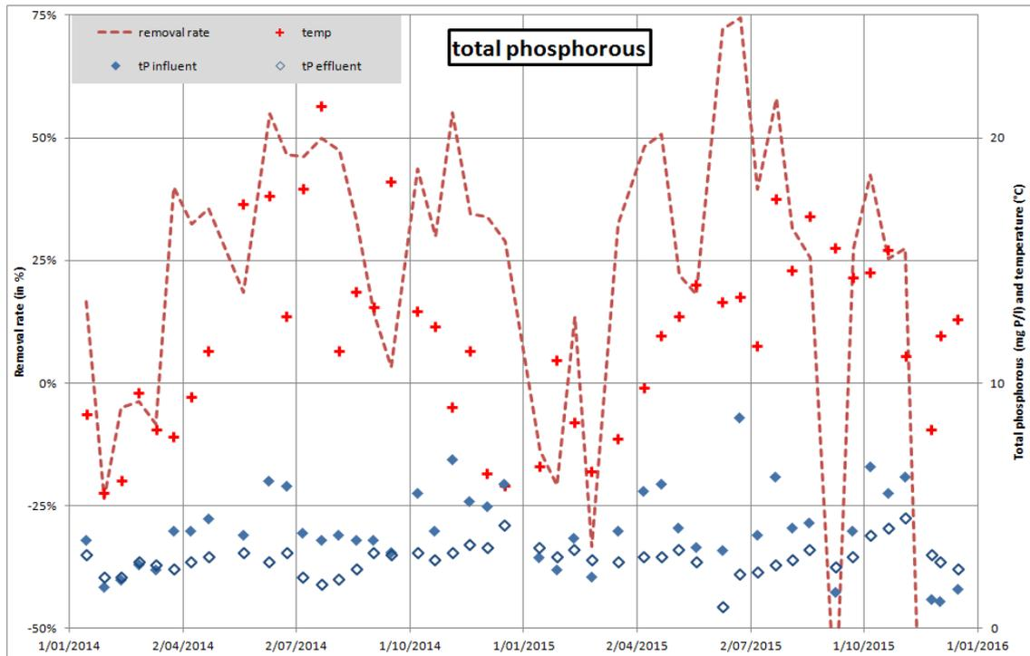
Figure 9 Concentration of total phosphorous in in- and effluent of willow field during 2014-2015
