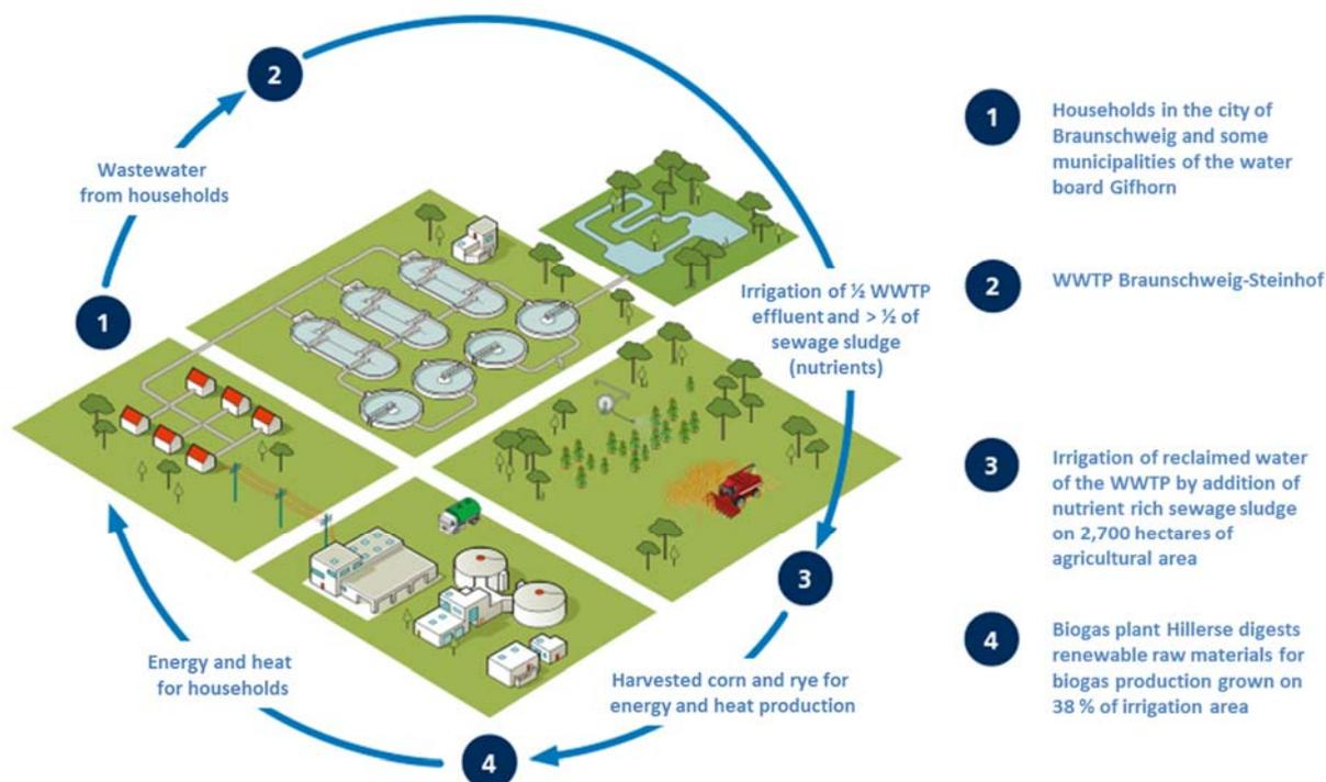
**Figure 16** The Braunschweig model of local water and nutrient recycling (simplified)
