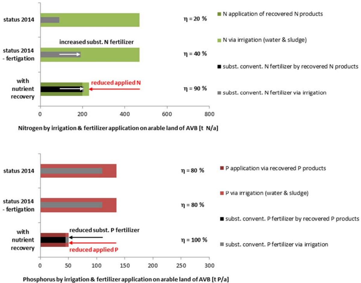
Figure 24 Total nitrogen and phosphorus input by irrigation and secondary fertilizer application on arable land of the AVB and effectiveness of applied nutrients regarding mineral fertilizer substitution (reuse-site perspective)
