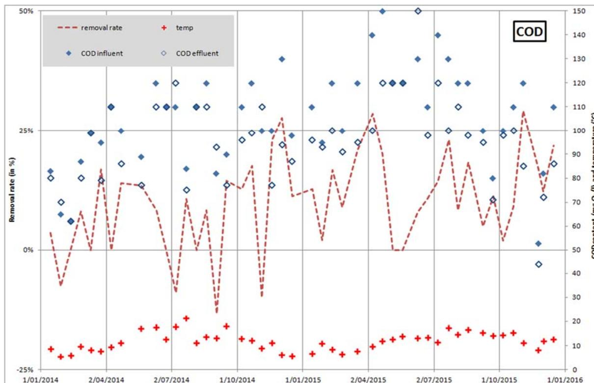
Figure 7 COD concentration in in- and effluent of willow field during 2014-2015
