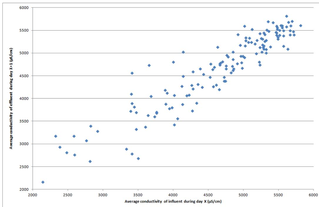
Figure 5 Relation between daily conductivity of influent and effluent the day after
