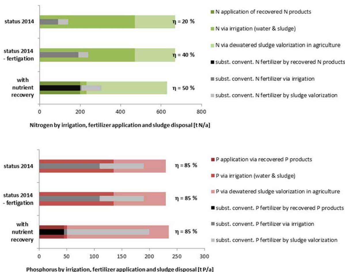
Figure 25 Total nitrogen and phosphorus input by irrigation and secondary fertilizer application on arable land of the AVB, nitrogen and phosphorus by agricultural valorisation of sewage sludge and effectiveness of applied nutrients regarding mineral fertilizer substitution (total perspective on nutrient valorisation)
