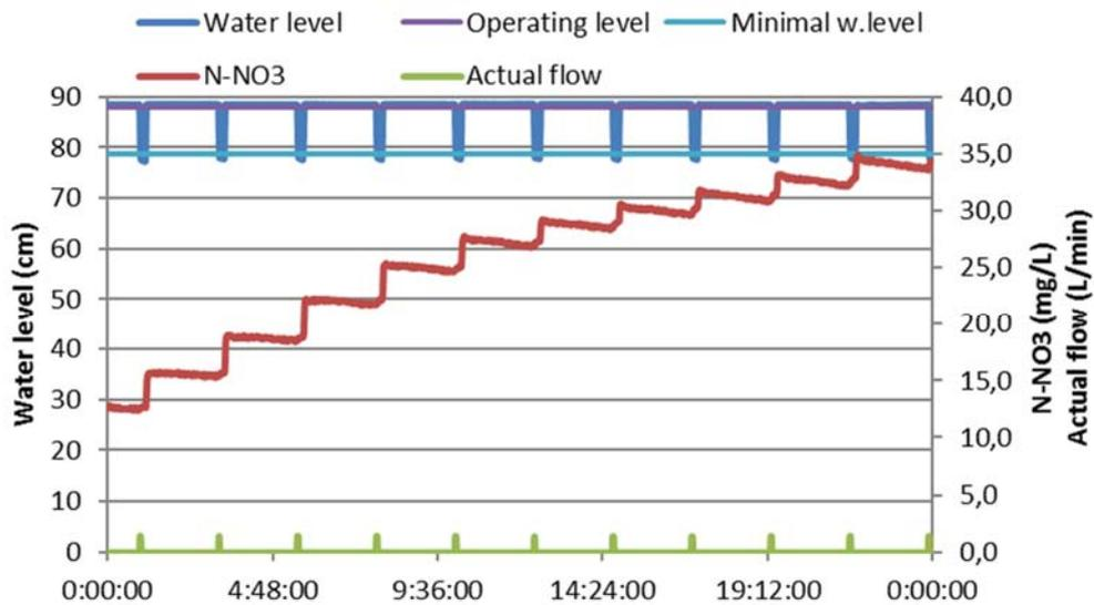
Figure 11 Nitrogen concentration, flow and water level of pilot MBBR – 13th December 2015
