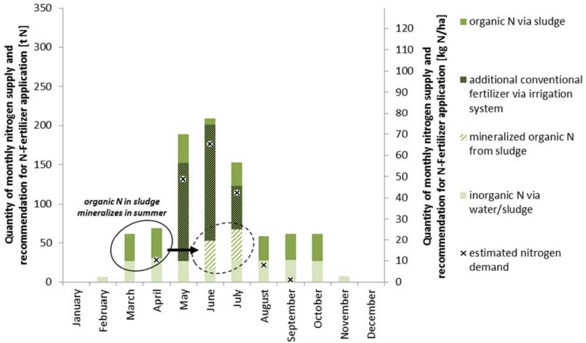
Figure 20 Adapted management of nitrogen fertilizer in the fertigation concept (data from 2014, and estimates)
