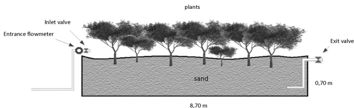
**Figure 2** Scheme of the willow-test field (Sept. 2013 – 2015)
