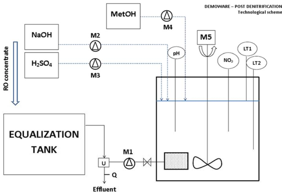
Figure 3 Technological scheme of post-denitrification MBBR
