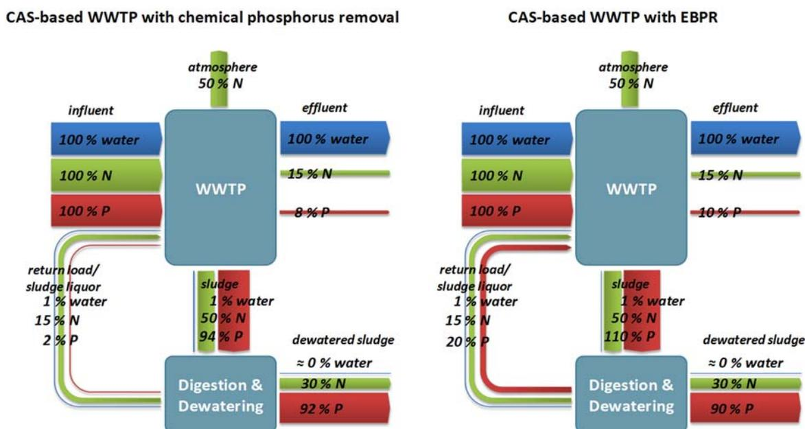
Figure 15 Averaged distribution of water, nitrogen and phosphorus flows in CAS-based WWTP with chemical phosphorus removal and EBPR (% relate to 100 % in WWTP influent)
