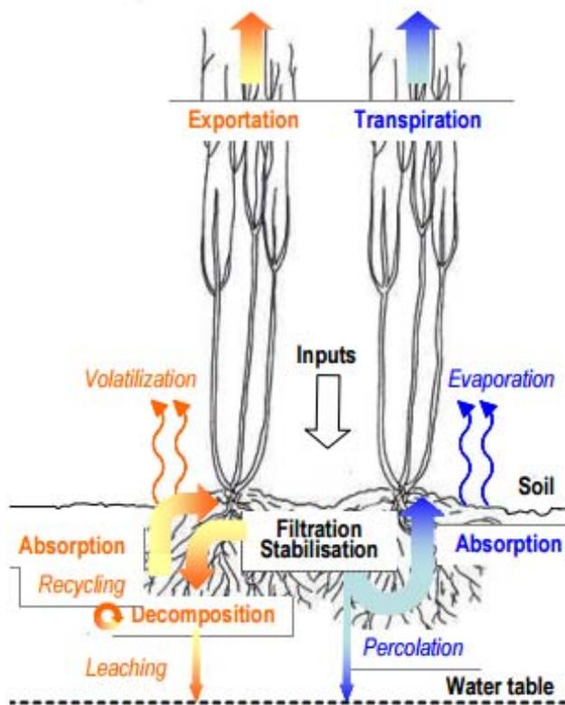
Figure 1 : Water and nutrient cycles in a SRWC
