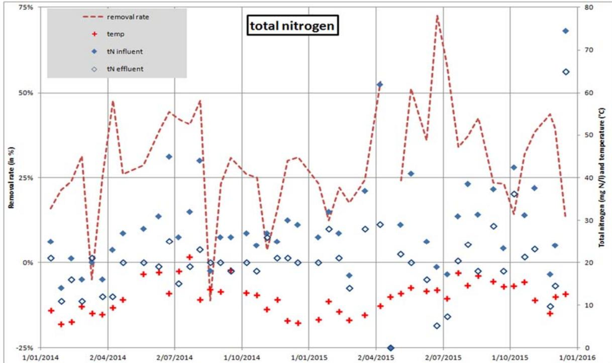
Figure 8 Concentration of total nitrogen in in- and effluent of willow field during 2014-2015
