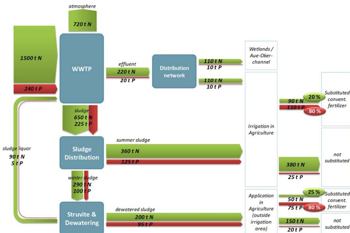
Figure 19 annual nutrient flows of the Braunschweig reuse scheme and currently substituted fertilizers
