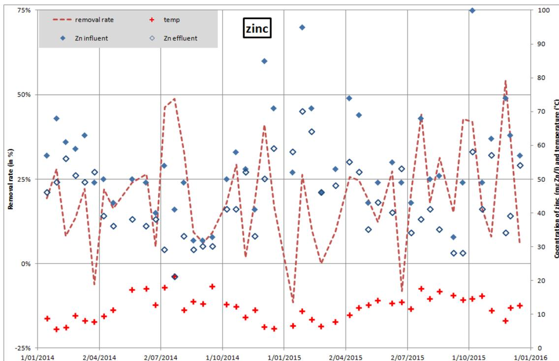
Figure 10 Concentration of zinc in in- and effluent of willow field during 2014-2015
