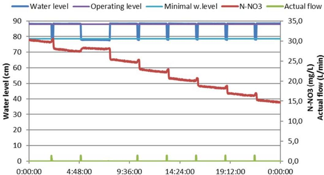
Figure 12 Nitrogen concentration, flow and water level of pilot MBBR – 16th December 2015
