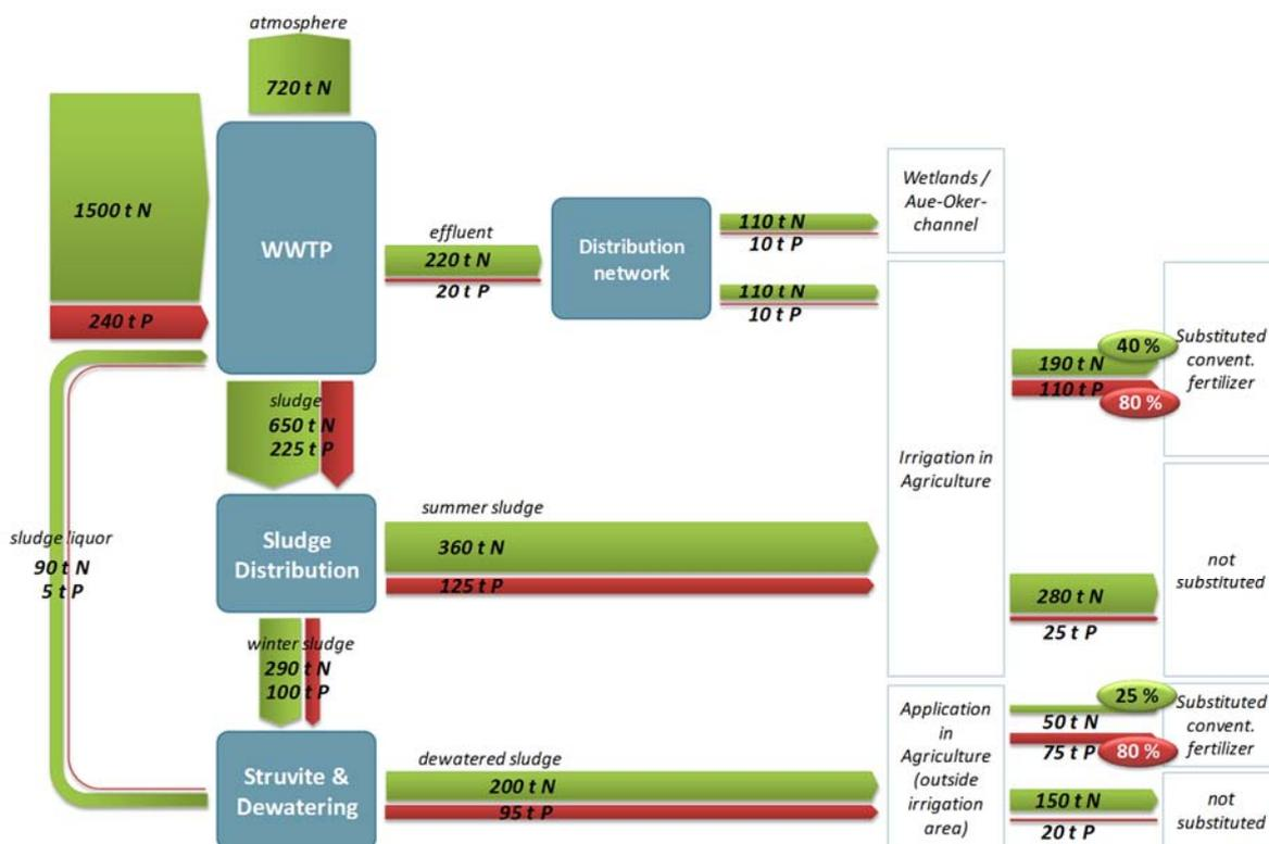
Figure 21 annual nutrient flows of the Braunschweig reuse scheme and substituted fertilizers in the fertigation concept
