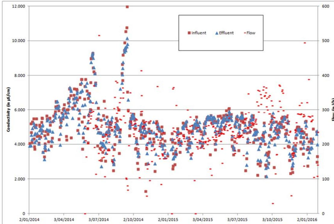
Figure 4 Average daily conductivity of in- and effluent of willow field and flow of the field
