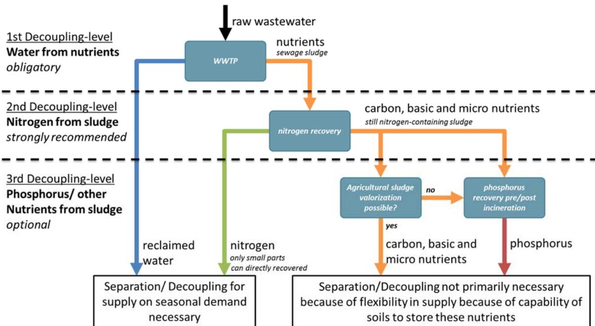
Figure 26 Three levels of decoupling nutrient and water management
